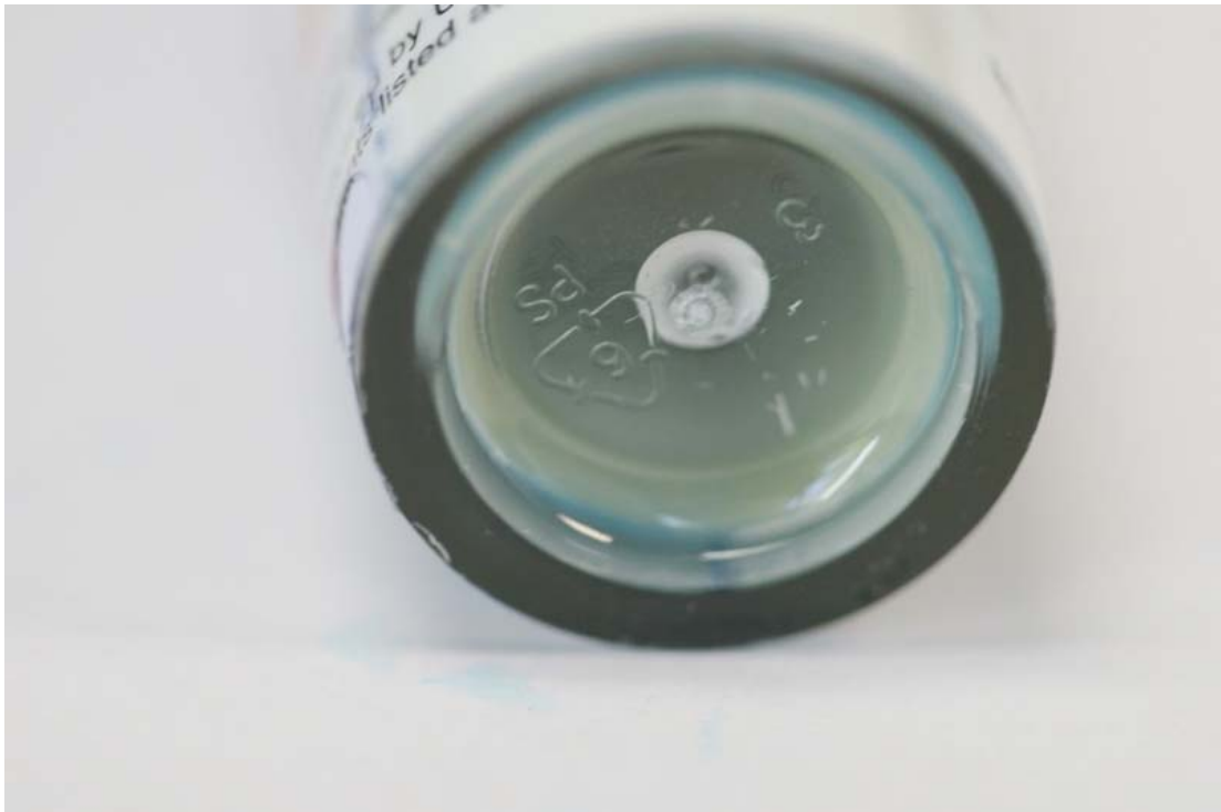
Sample #7 after dye penetration test
