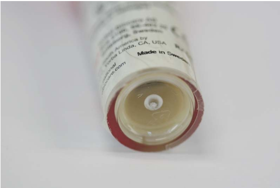
Sample #1 before dye penetration test
