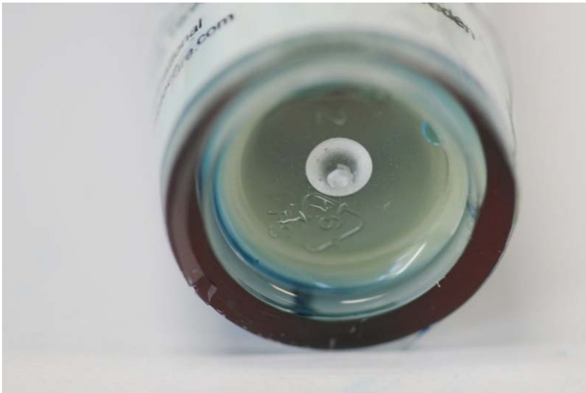
Sample #6 after dye penetration test
