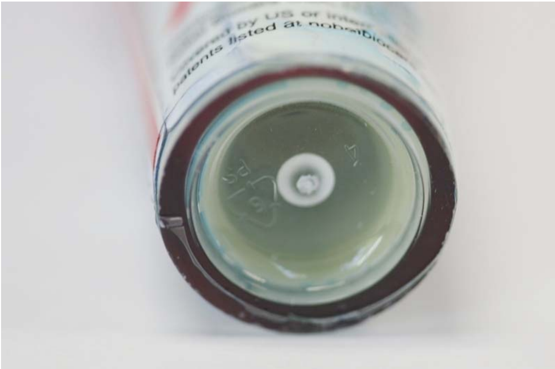
Sample #1 after dye penetration test
