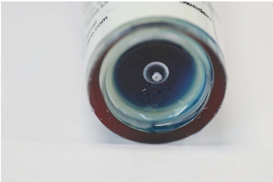
Sample #5 after dye penetration test
