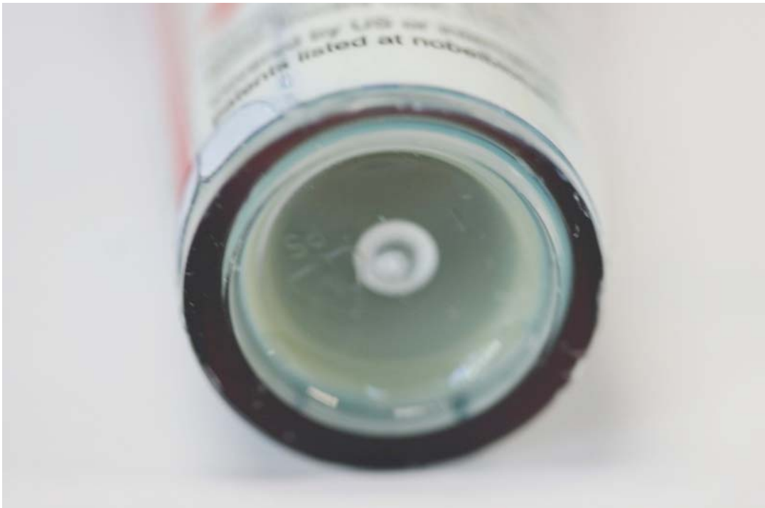
Sample #2 after dye penetration test
