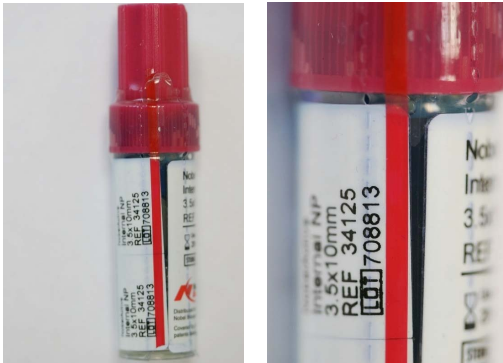
Sample #1 after dye penetration test
