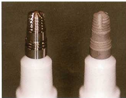
Fig. 1. Machined and etched implants as used in the study.
