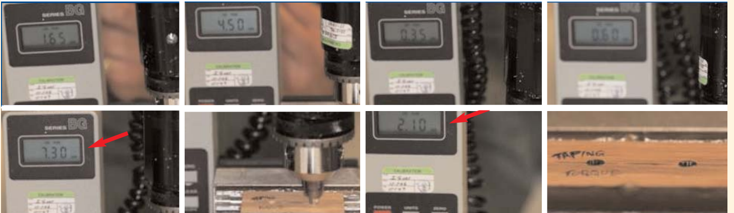
RePlant 4.3mmD/10mmL Insertion Torque Insert Implant 1/4mm Above Pre-tapped hole in Oak Required 2.35in/lb (26.55Ncm)
