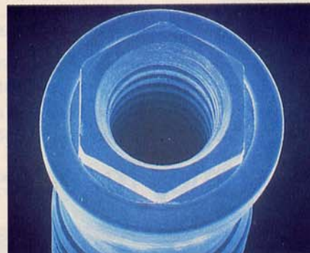
Figure 4—Scanning electron micrograph of external hex connection with flat shoulder for abutment support.
