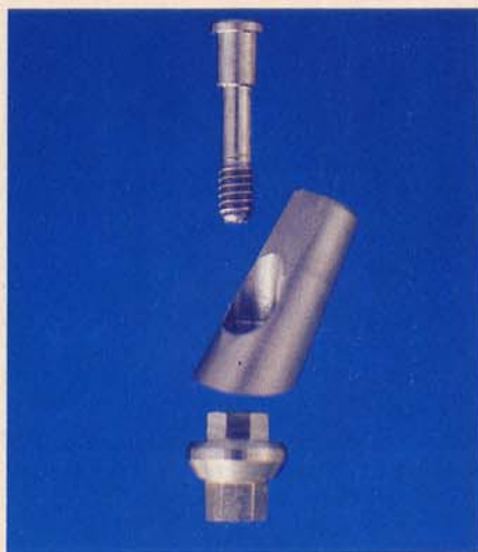
Figure 7—30 degree Preangled Tapered Abutment with intermediate hexagon/octagon base and fixation screw allows 24 adjustments every 15 degrees.
