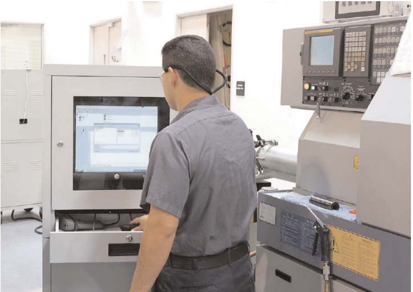
Jesus Guillen, setup machinist, uses Shop Floor Automation's Predator DNC software to download a program to one of Implant Direct's 26 Star turning centers.
