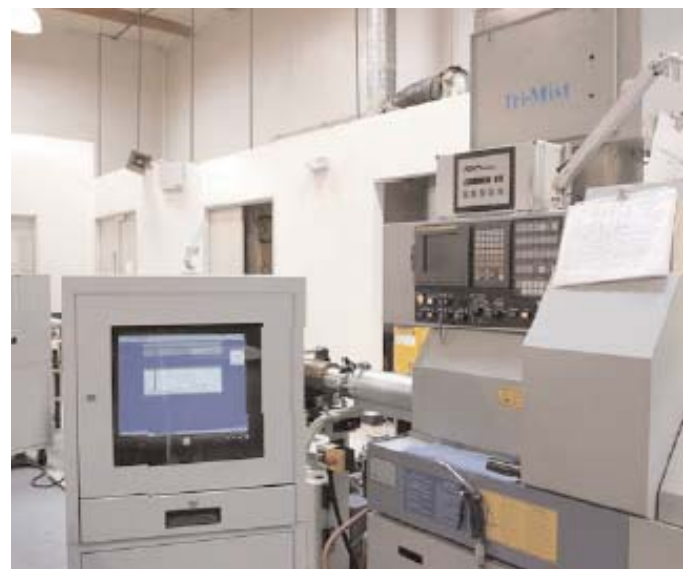
Atam throughput optimization system at work. The Atam, a black box sitting on top of the Star, monitors system vibration and yields reports as required.
