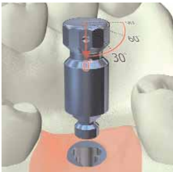
Dimple of Alignment Tool is perpendicular to labial: 0 degree offset of implant tri-lobe.
